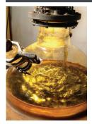
**Hydroalcoholic extractions** use water and alcohol to remove the alcohol soluble compounds from essential oils and related products. This process was developed to address the needs of a number of industrial applications, including those in the citrus juice industry. The citrus fruit harvest can be optimized by utilizing the peel and
