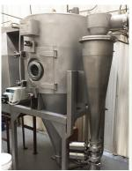
slightly different proportions of water, gums, and flavor materials. Flavor encapsulation can be achieved through a process known as spray drying. Spray drying is the conversion of liquid, usually oil soluble, into a water dispersible fine powder.
